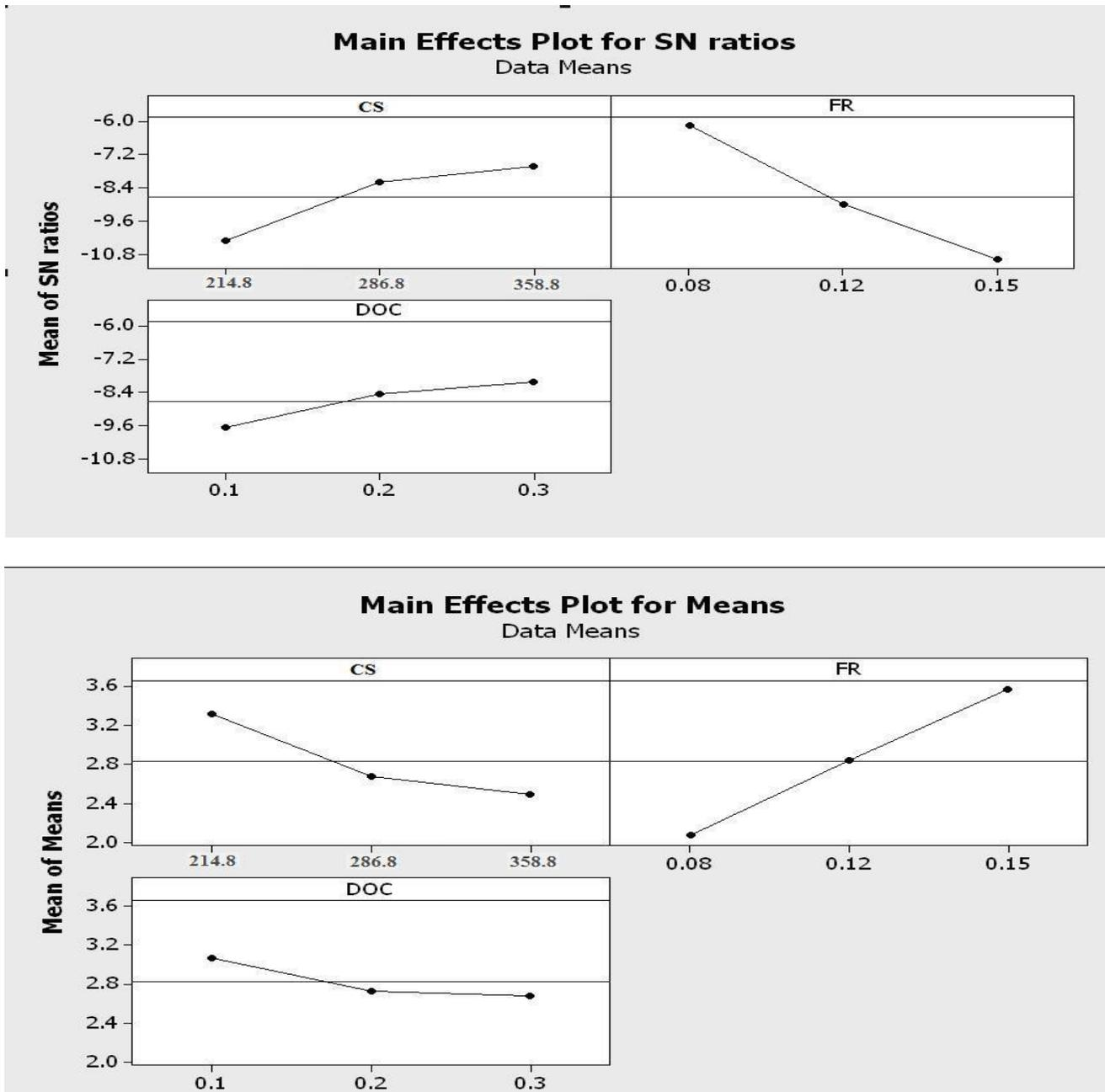
Figure 3 Main effects plot for SN ratios and mean (surface roughness)
