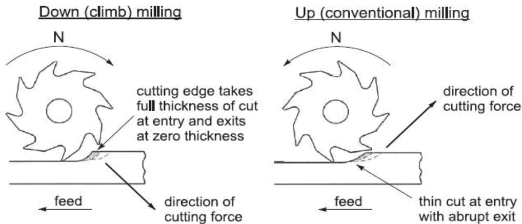
fig.3 types of milling process
