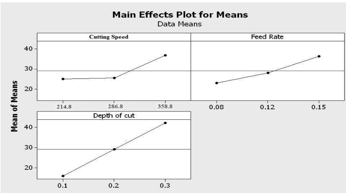
Figure 4. Main effect plots for SN ratio and mean data (MRR)
