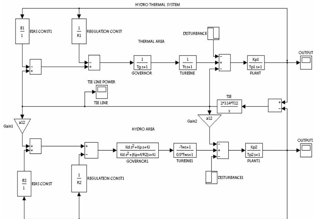
Fig. 5, Mathematical model of Hydro-Thermal System
