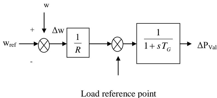
Fig. 2 Transfer function model of Governor
