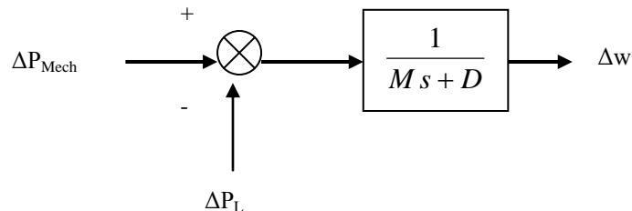
Fig. 4 Transfer function model of Generator-load
