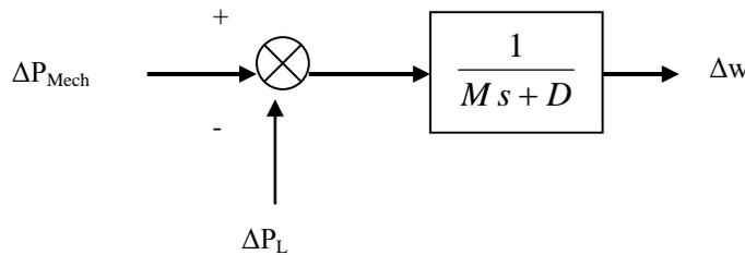
Fig. 4 Transfer function model of Generator-load
