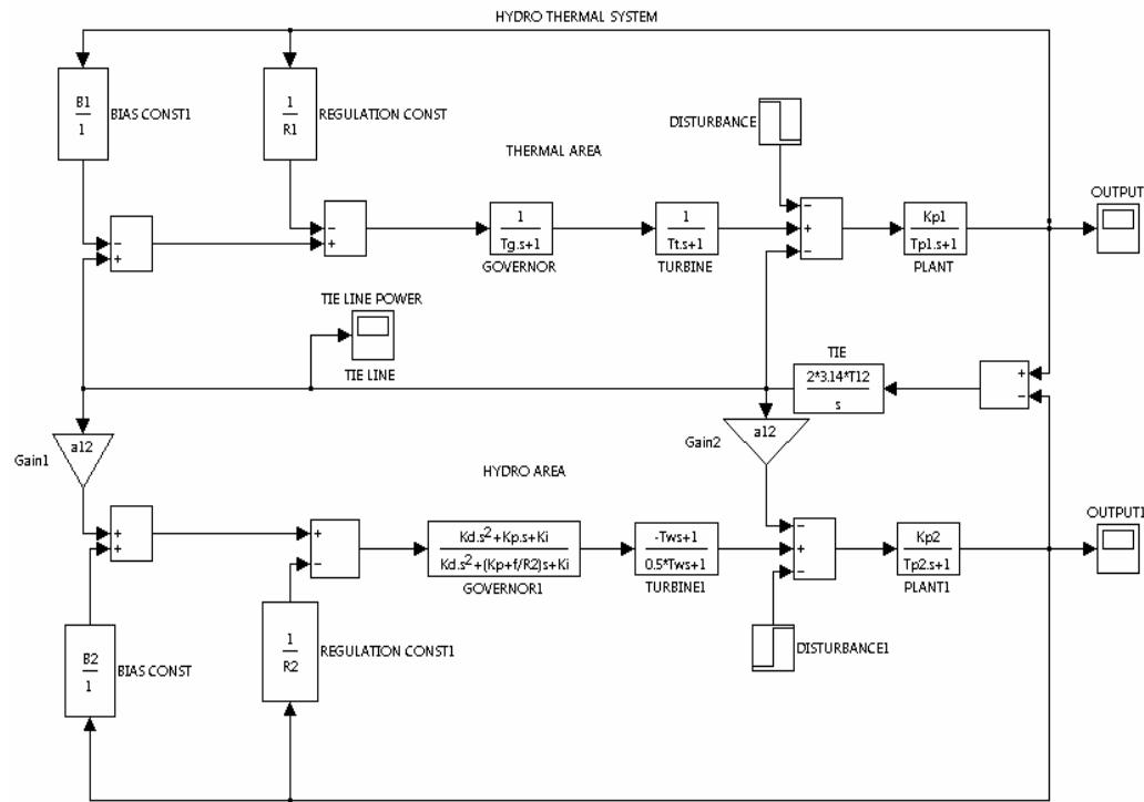
Fig. 5, Mathematical model of Hydro-Thermal System
