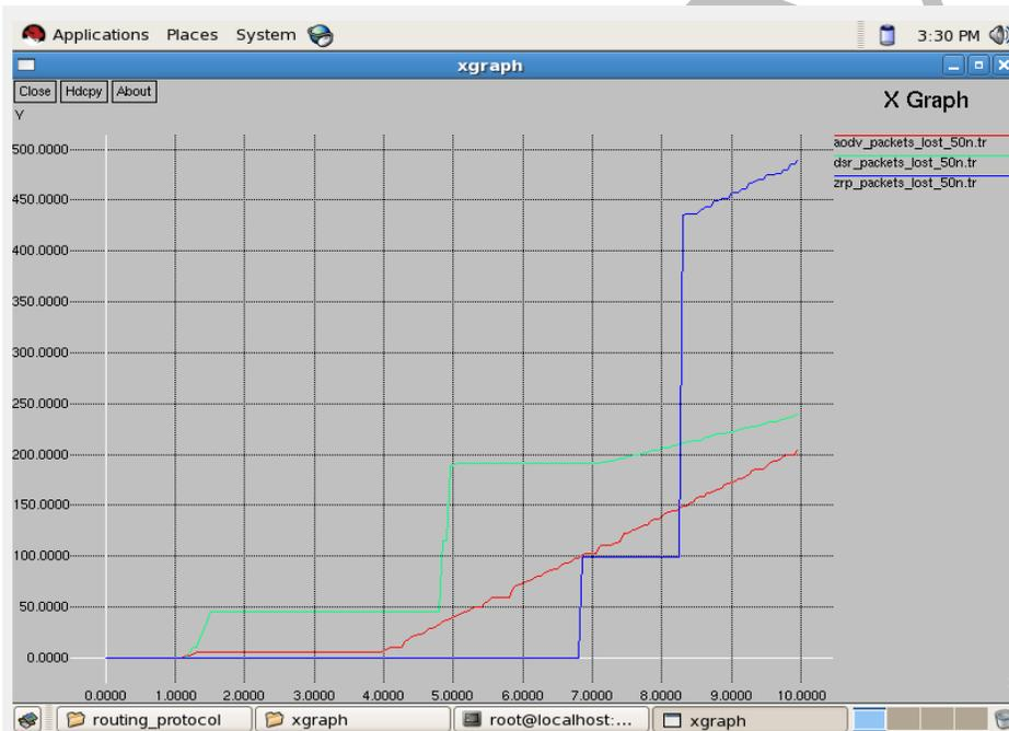
Fig 9: X-graph representing comparison of packet lost in simulation for AODV, DSR and ZRP. In fig 9, the number of packets lost in ZRP is much higher than other routing protocols. Packets lost is minimum in case of AODV.
