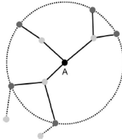
Fig.7 ZRP - Routing Zone of Node A  $\rho= 2$  (adapted from [2])
