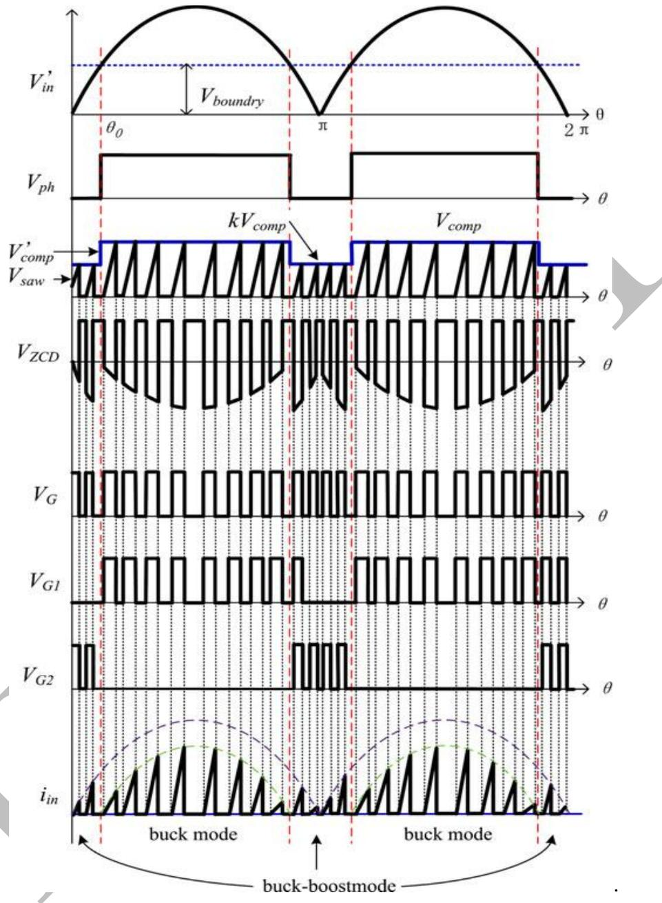
Fig. 6. Key waveforms of rms in the improved COT control diagram.
