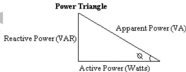
Fig.2: Harmonic distortion and Power factor triangle
