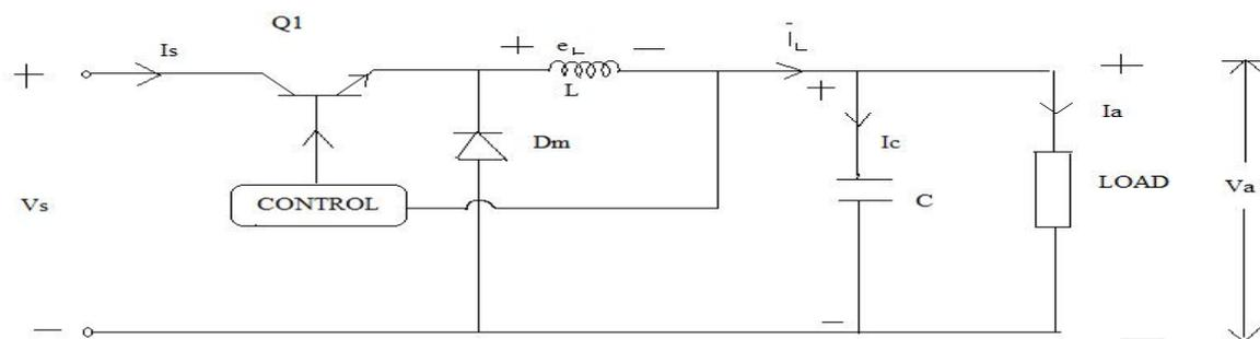
Fig 1. Circuit Diagram of Buck Converter
