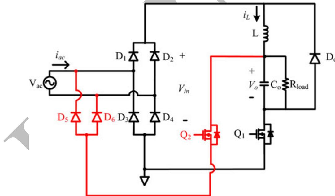
**Fig. 3.** Improved buck PFC converter.
