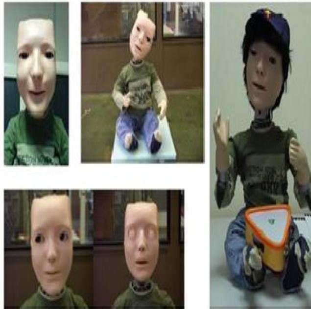
Figure1. The minimally expressive humanoid robot KASPAR designed for social interactions
