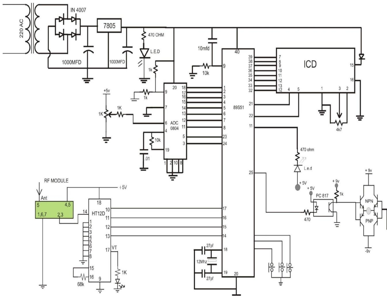
**Fig.2 Circuit Diagram for Speed Control**
