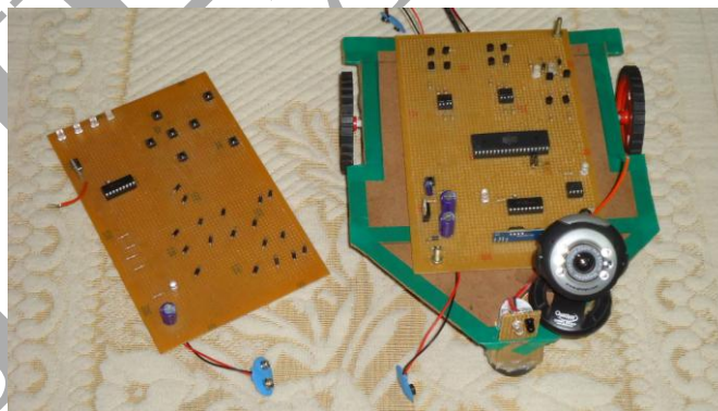
Fig---RF ROBO WITH WIRELESS CAMERA
