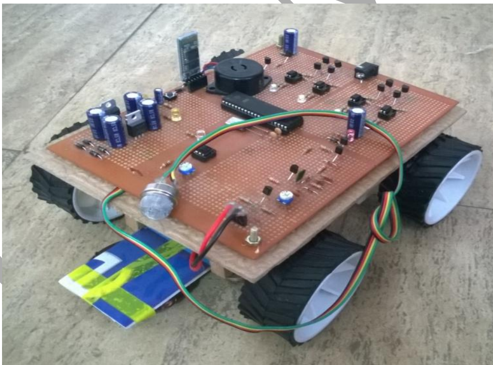
Fig 2: Prototype Design of Landmine and Gas Detector Using Android
