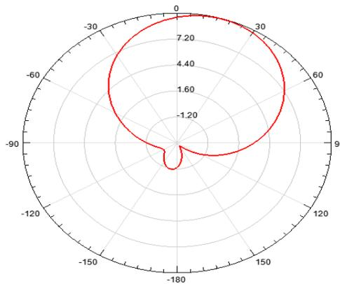
**FIGURE 12-RADIATION PATTERN AT  $\phi=0$  AND AT FREQUENCY=6 GHz**
