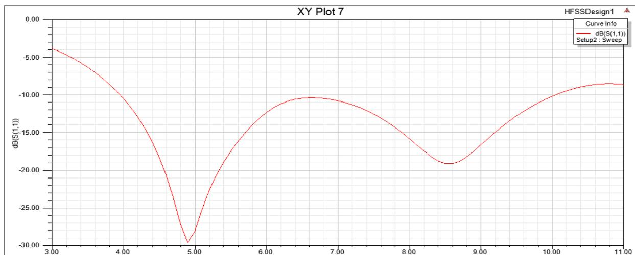
**FIGURE 7-THE RETURN LOSS CHARACTERISTICS (S11 PARAMETERS) OF THE ANTENNA WITH THE DESIGN 2**
