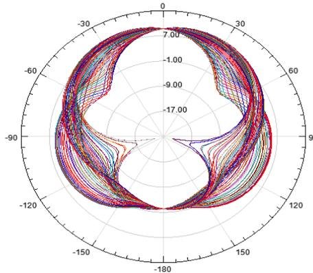
FIGURE 9-RADIATION PATTERN AT ALL  $\phi$  AND AT FREQUENCY=6 GHz
