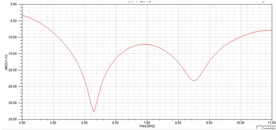
**FIGURE 11-THE RETURN LOSS CHARACTERISTICS (S11 PARAMETERS) OF THE ANTENNA WITH THE DESIGN1**
