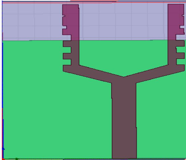
**FIGURE 6- THE PROPOSED ANTENNA IN HFSS SOFTWARE.(TOP VIEW) WITH SLOTS OF DESIGN 2**
