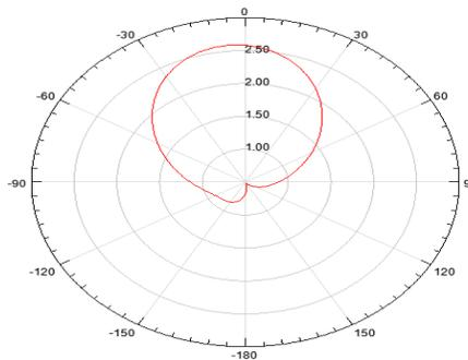
**FIGURE 4-RADIATION PATTERN AT  $\phi=0$  AND AT FREQUENCY=6 GHz**
