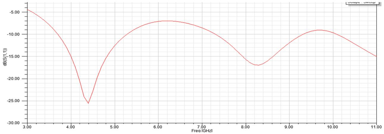
**FIGURE 3-THE RETURN LOSS CHARACTERISTICS (S11 PARAMETERS) OF THE ANTENNA WITH THE DESIGN1**
