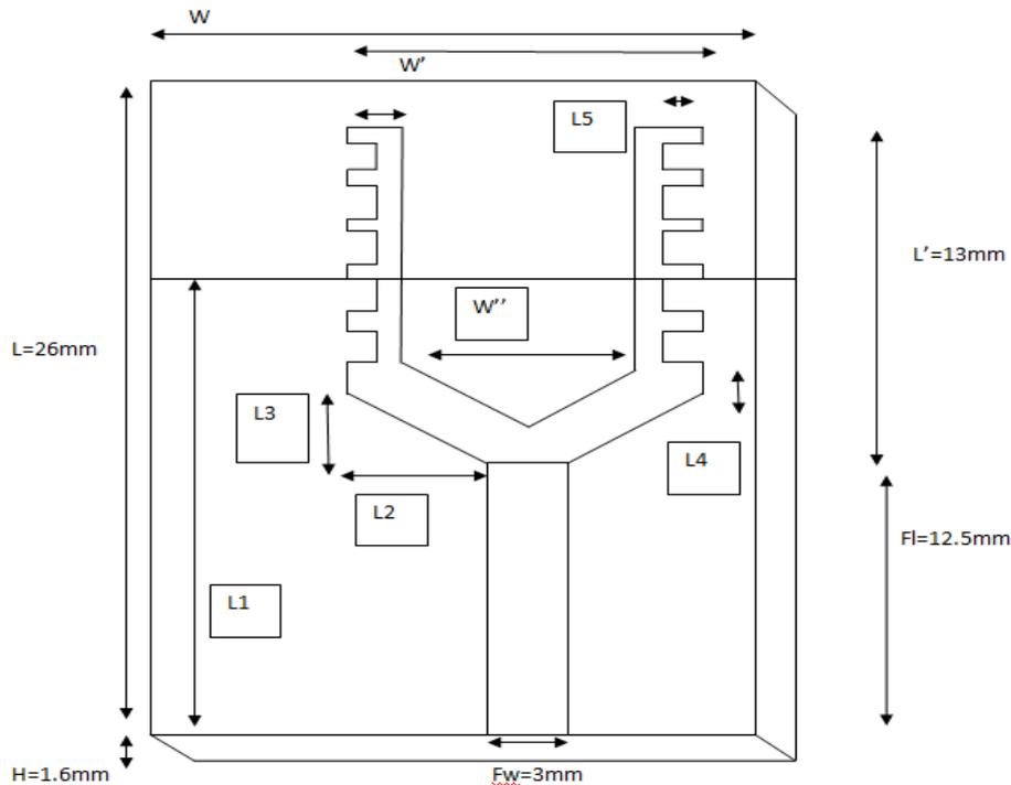
L1=19.5mm L2=7mm L3=2mm L4=2mm L5=1.5mm W''=11mm W'=15mm W=23mm
