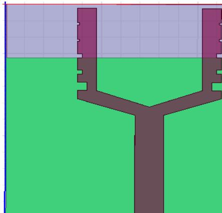
FIGURE 10- THE PROPOSED ANTENNA IN HFSS SOFTWARE.(TOP VIEW) WITH SLOTS OF DESIGN 3
