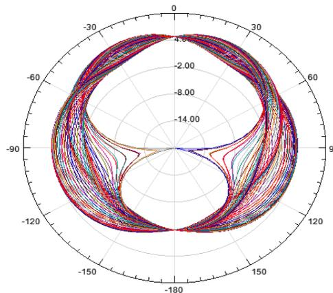
**FIGURE 5-RADIATION PATTERN AT ALL  $\phi$  AND AT FREQUENCY=6 GHz**
