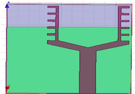
FIGURE 2- THE PROPOSED ANTENNA IN HFSS SOFTWARE.(TOP VIEW) WITH SLOTS EQUALLY CUT OF DIMENSIONS 1.5mm\*1.5mm
