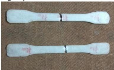
Figure 6. Sample with glass fiber + epoxy resin + SnO<sub>2</sub> after tension test
