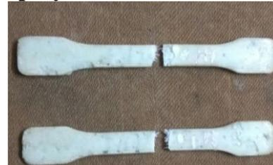
Fig 8. Sample with glass fiber + epoxy resin after tension test
