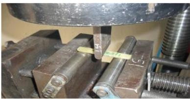
**Figure 12. Specimen during flexural test**
