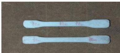
Figure 4. Sample with glass fiber + epoxy resin before tension test
