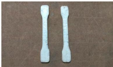
Figure 5. Sample with glass fiber + SnO<sub>2</sub> + epoxy resin before tension test
