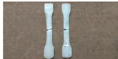
Figure 9. Sample with glass fiber + PTFE + epoxy resin after tension test
