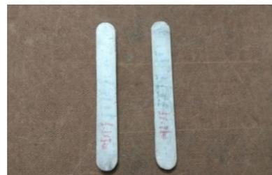
**Figure 15. Sample with glass fiber + SnO<sub>2</sub> + epoxy resin before flexural test**
