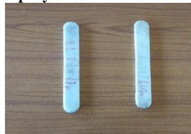
**Figure 16. Sample with Fiber + epoxy resin + PTFE powder before flexural Test**
