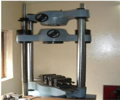
**Figure.10. UTM for Flexural test**
