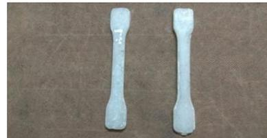
Fig 7. Sample with glass fiber + PTFE+ epoxy resin before tension test
