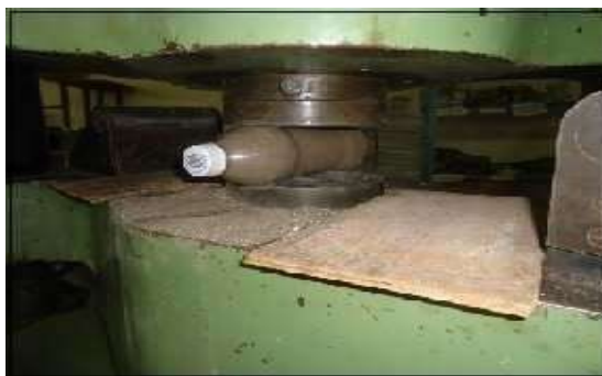
Fig. 8. Test applied on a waste PET bottles filled with soil and sealed tightly
