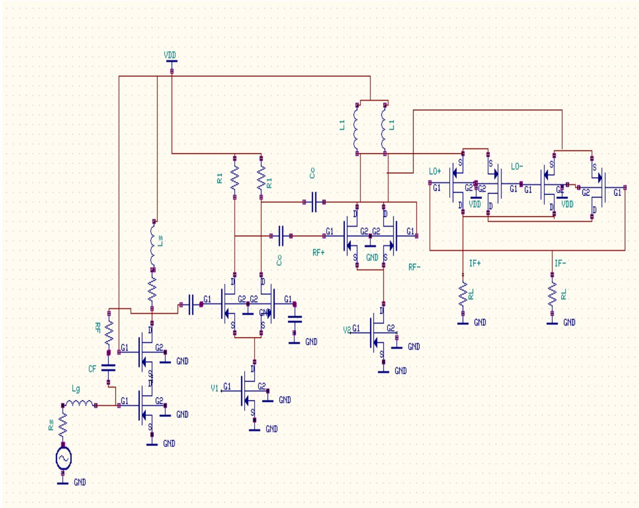
**Figure 1 Novel High Gain Receivers**
