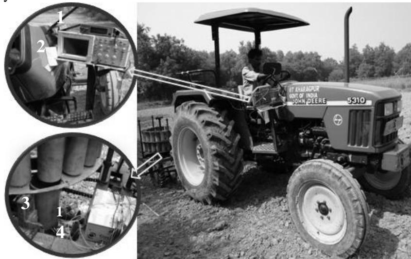
1. Seedling counter 2. Oscilloscope 3. Optoelectric sensor 4. Optical sensor box
