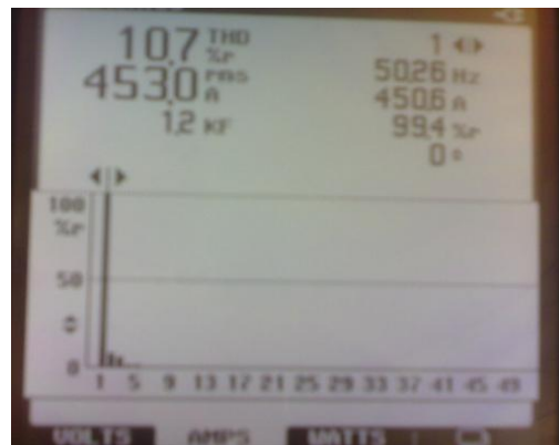
Figure 18. THD analysis using power quality analyzer
