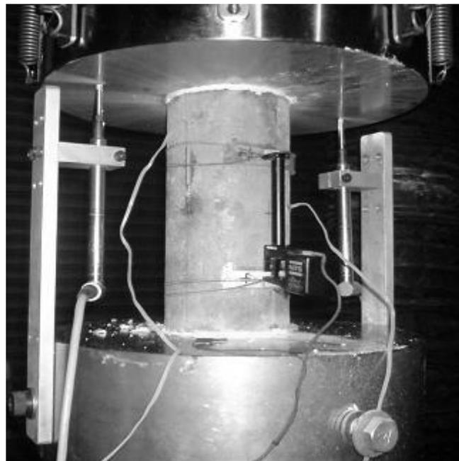
**Figs-1 & 2 Experimental set up for cylinders under uniaxial compression**
