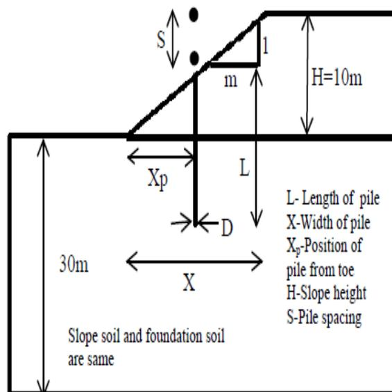
Figure 1 Geometry of the pile slope system
