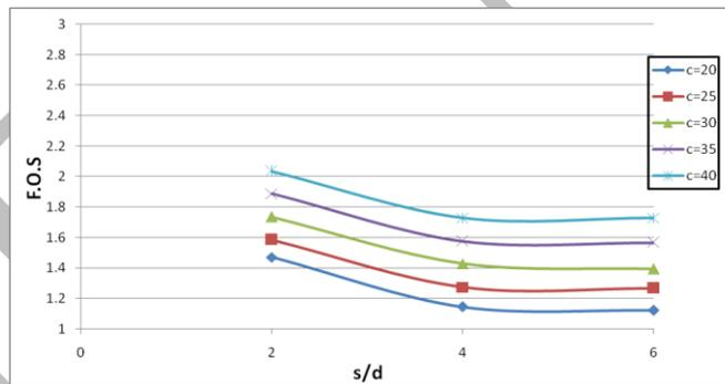
**Figure 7** Variation of safety factor with respect to the s/d ratio for clayey soil slope
