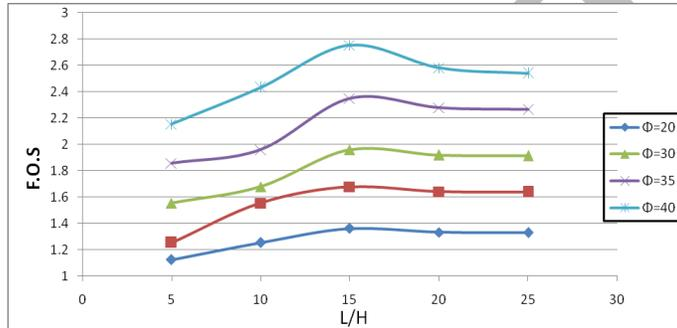
**Figure 6** Variation of safety factor with respect to the length of the pile for sandy soil slope
