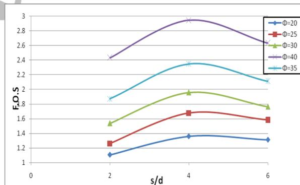
**figure 8** variation of safety factor with respect to the s/d ratio for sandy soil slope
