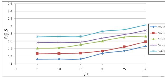
**Figure 5** Variation of safety factor with respect to the length of the pile for clayey soil slope
