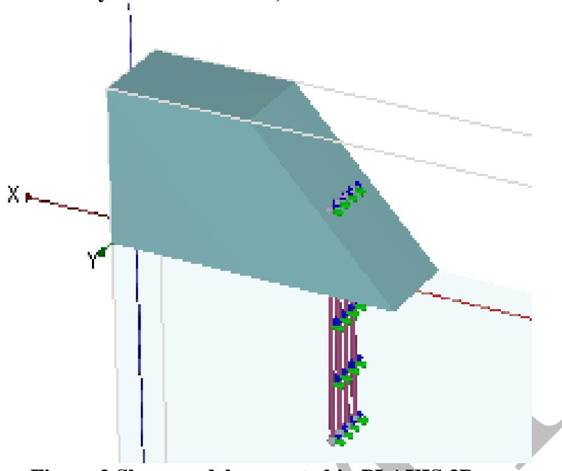
Figure 2 Slope model generated in PLAXIS 3D
