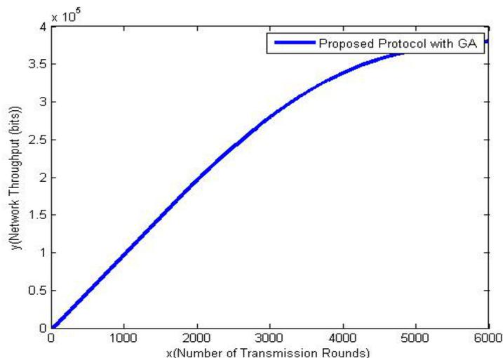
**Fig 6. Network throughput with respect to number of rounds for the proposed protocol with GA**
