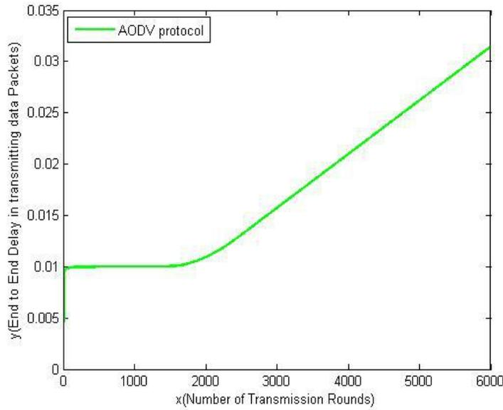
**Fig.7 End-to-End delay for the AODV with respect to number of rounds**
