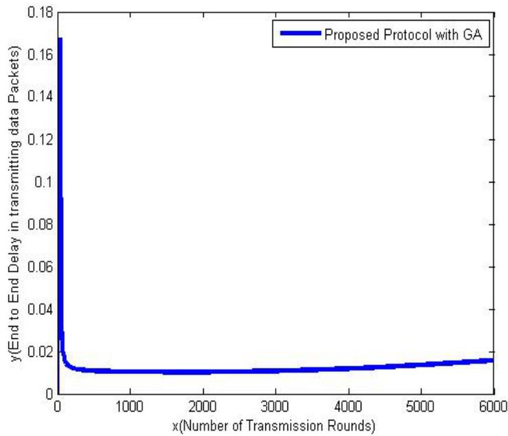
**Fig 8. End-to-End delay with respect to number of rounds for the proposed protocol with GA**
