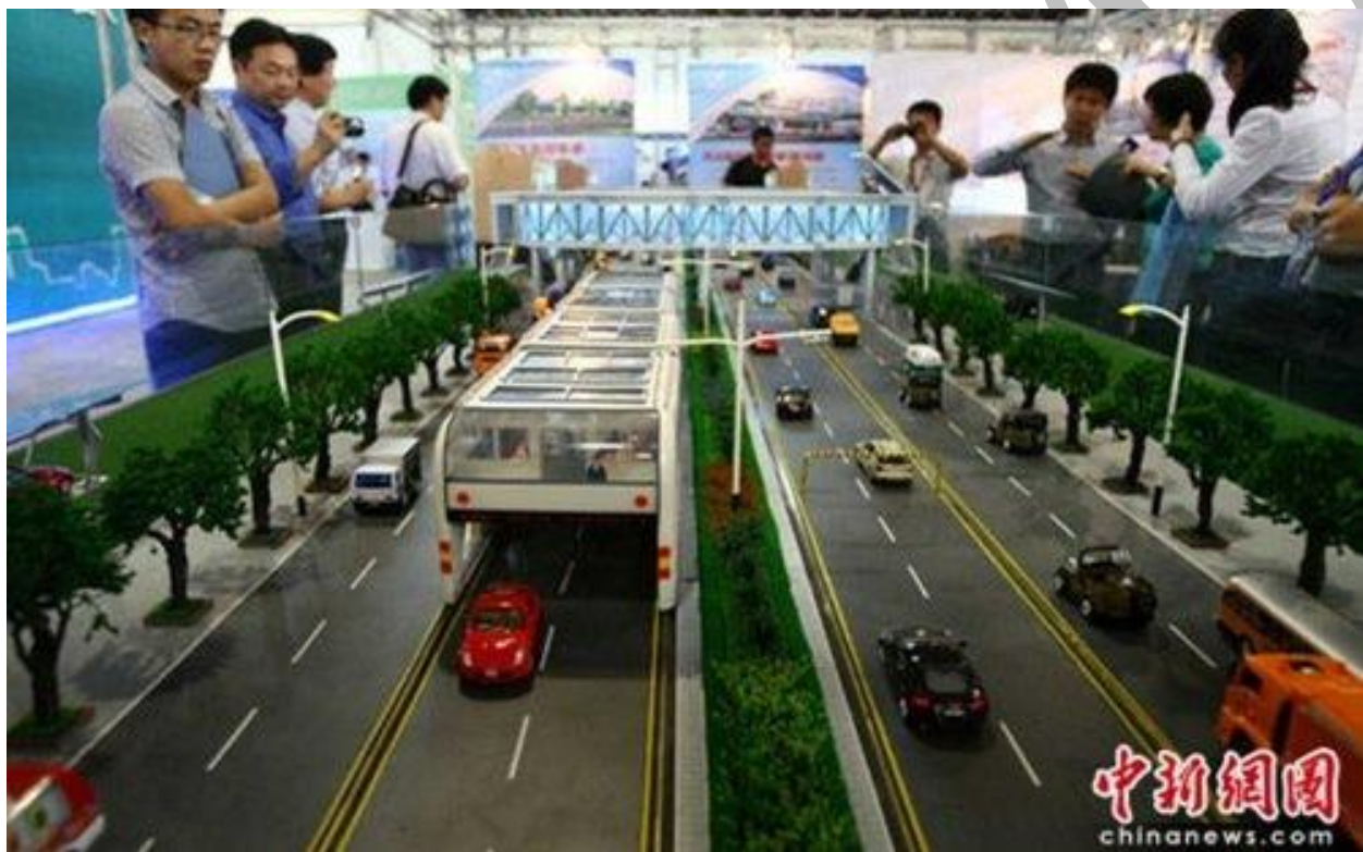
Fig. 2: Showing the model of the Straddling Bus
